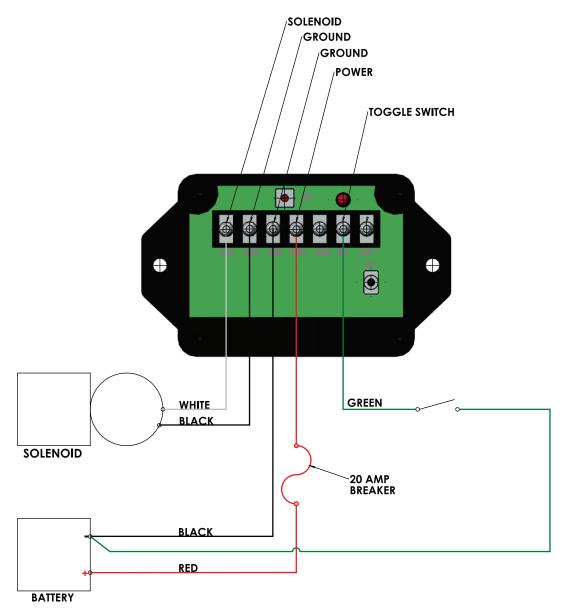
Power and ground MUST be run directly back to the battery with 14 gauge wire (maximum 9.5'). Improper grounding will cause damage to the component, voiding warranty.
