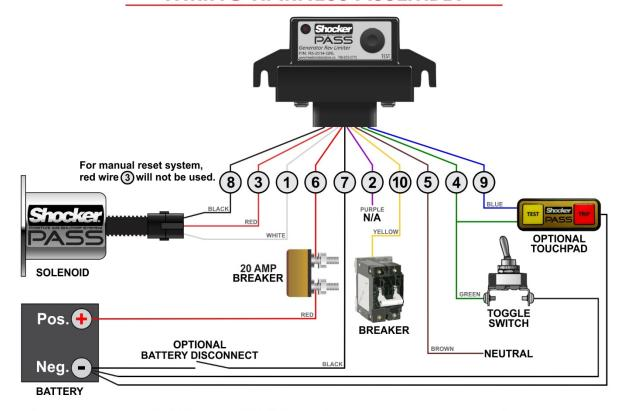
Power and ground MUST be run DIRECTLY to the battery with a minimum of 12 gauge wire. Improper grounding WILL cause damage to the component, voiding warranty.
