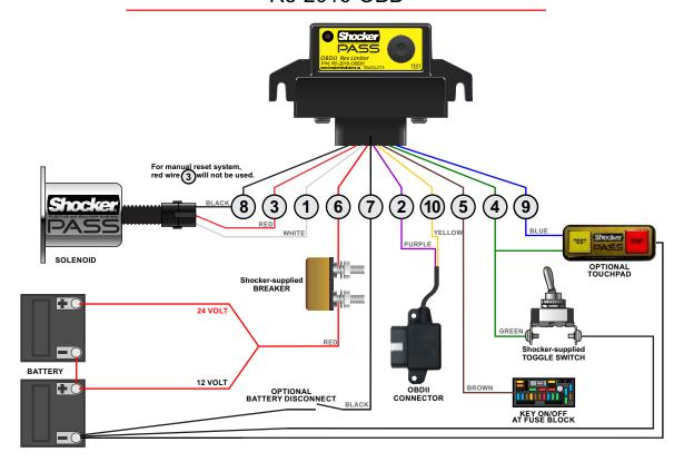
Use crimp-type heat shrink connectors. Power and ground MUST be run DIRECTLY to the battery with a minimum of 12 gauge wire. Improper grounding WILL cause damage to the component, voiding warranty.
