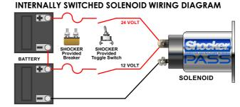
Use crimp type connectors & heat shrink tube on both 12V and 24V Solenoids. WIRE SIZE RECOMMENDATION TABLE
