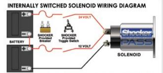
Use crimp type connectors & heat shrink tube on both 12V and 24V Solenoids.
